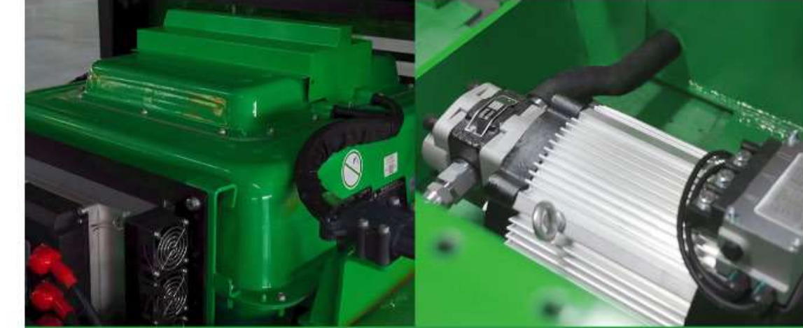
New Lithium-ion Battery and Motor
